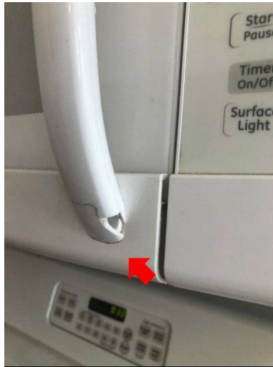
Microwave handle is damaged
